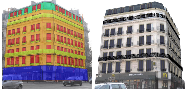
Figure 10. 3D reconstruction of a building with multiple facades visible from the street. Note that floors align seamlessly along the different facades.
